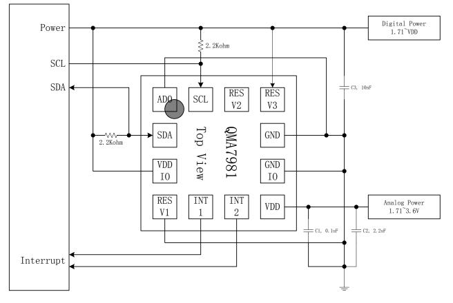
Figure 5. Dual Supply Connection
