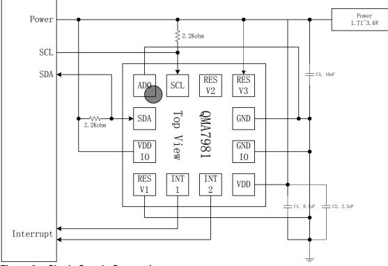
Figure 6. Single Supply Connection
